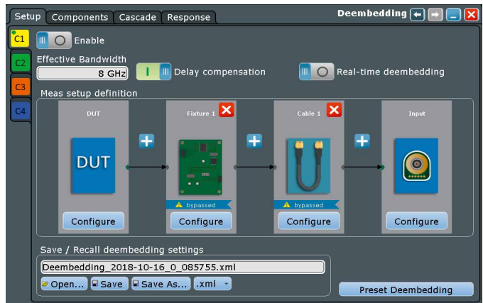
Fig. 3: Signal path configuration with transmission components between the DUT and the oscilloscope input.
