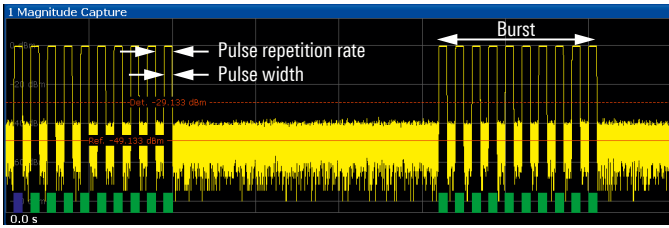
Fig. 2: Burst signal: ten pulses are followed by a longer pause up to the next burst.
