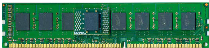
Fig. 20: DIMM with interposer for using a solder-in probe tip module to contact DDR3 signals.
