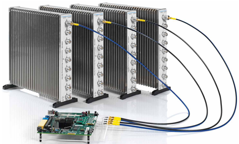
Fig. 5: The true MIMO TX measurement requires a separate R&S®CMW100 for each MIMO antenna. A control and evaluation PC for managing the test sets is always required (not shown here).
