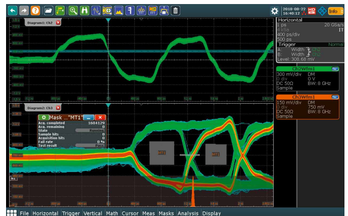
Fig. 2: Eye diagram of DDR3 write cycles with mask test and histogram.
