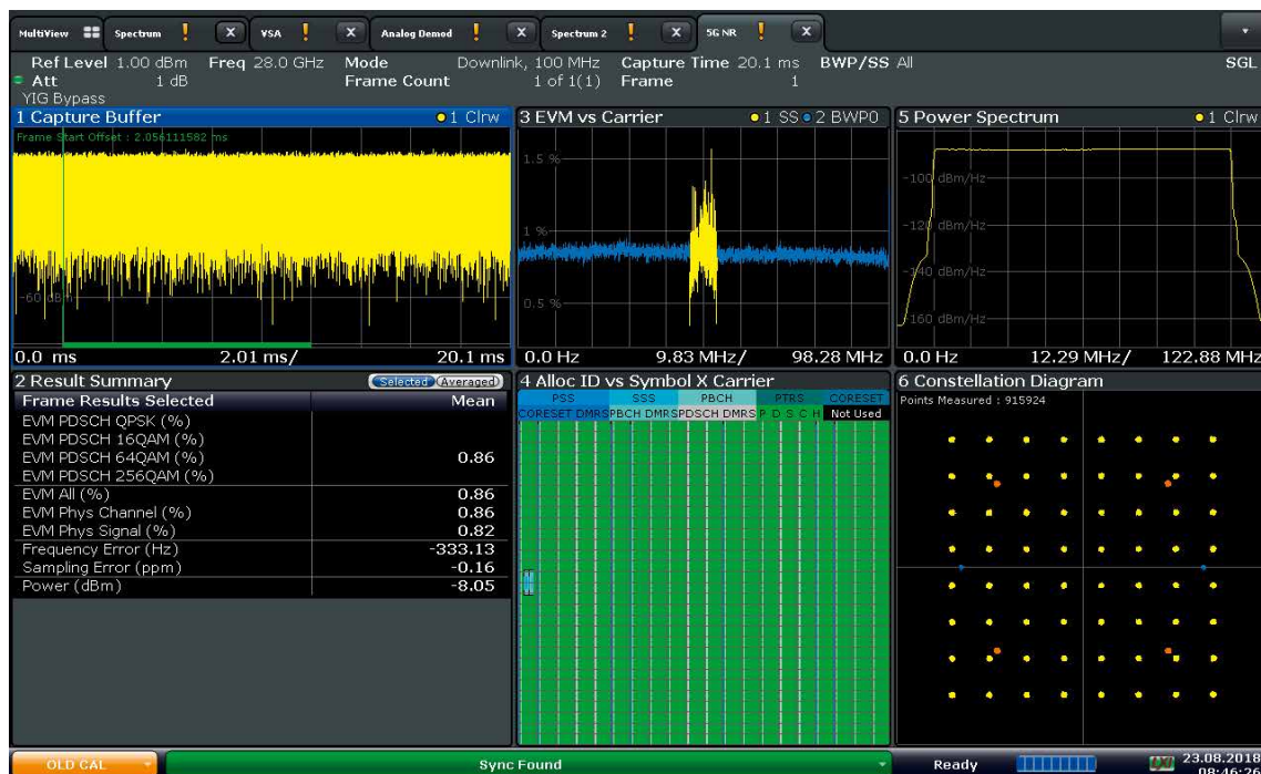
Fig. 3: Analysis of a 5G NR downlink signal at 28 GHz with the R&S®FSW-K145 option. Various views, such as EVM vs. carrier, the constellation diagram and tabular listing of all important parameters enable fast characterization or optimization of the 5G application.
