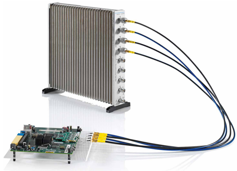
Fig. 4: Test setup for the switched MIMO TX measurement. Each antenna in the DUT is connected to a port on one R&S®CMW100. The ports are switched in rapid succession to the test set's analyzer.
