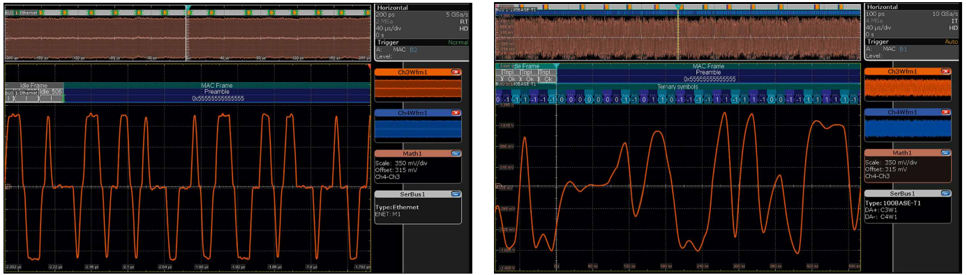
Fig. 2 On the left is a differential 100BASE-TX signal. The three levels and steep transition edges are clearly visible. An automotive 100BASE-T1 signal is shown on the right for comparison. Due to predistortion in the equalizer, the levels of the PAM-3 signal are not always clearly recognizable.
