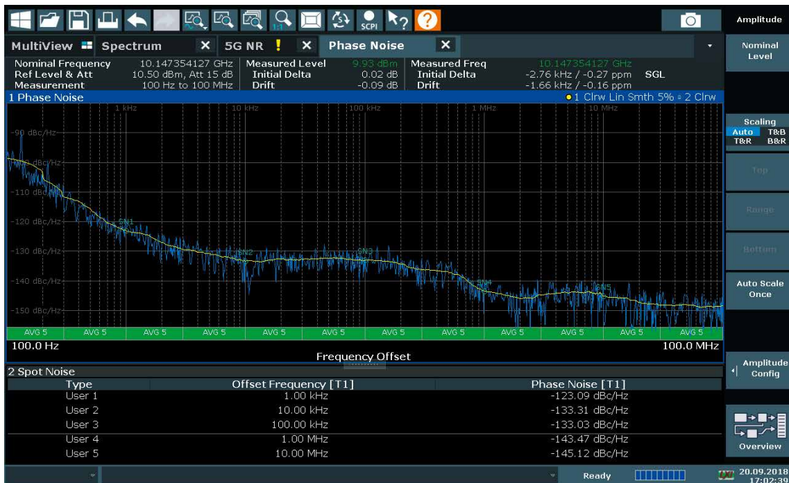
Fig. 5: Phase noise measurement on a high-grade oscillator at 10 GHz with the R&S®FSW-K40 measurement application. The measurement results for various offset frequencies are shown at the bottom.
