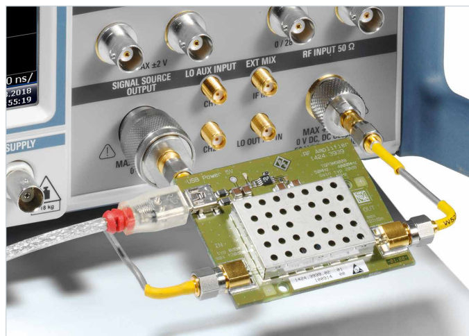
Fig. 1: Residual measurement of the phase and amplitude stability of pulses on an amplifier. The R&S®FSWP feeds the pulsed signal to the amplifier and analyzes the amplifier's output signal.
