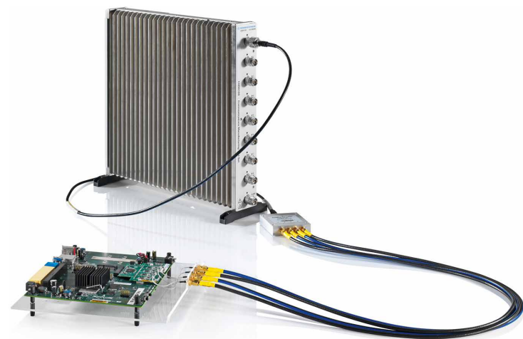
Fig. 2: Test setup for the composite MIMO TX measurement. A WLAN device with four antennas is connected to the R&S®CMW100 via a power combiner.
