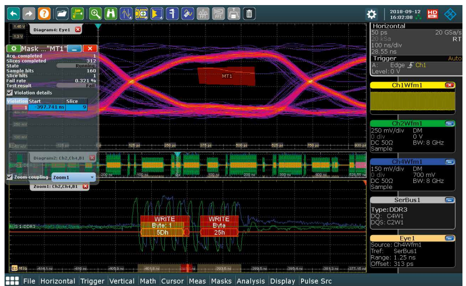
Fig. 10: Eye diagram of the write cycles with eye stripe marking of mask violations.
